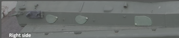
Two main embrasures for the infantry on board (both sides) and an additional square firing-hole (two on the left side)
