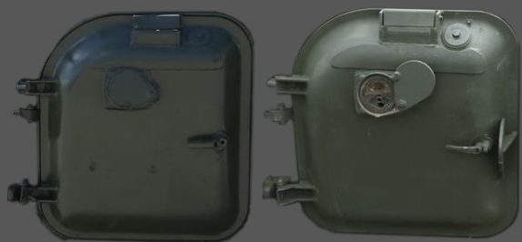
The rear dismant doors have two forms, one is shared with the BMP-1 (left) with the lever type , while on the modernised BMP-2's (right) with the shielded-lever type .
