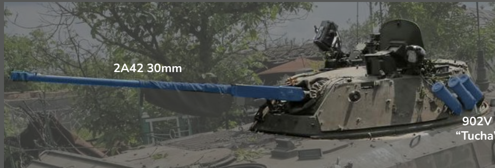
2A42 30mm autocannon is employed on a newer and wider turret to accompany two crew. Alongside, a pair of three 902V "Tucha" smoke launching tubes are on both sides of the turret.
