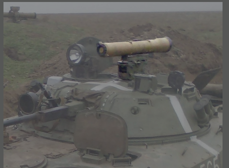
Launch rail and sight for the 9M113 Konkurs ATGM on the turret.
