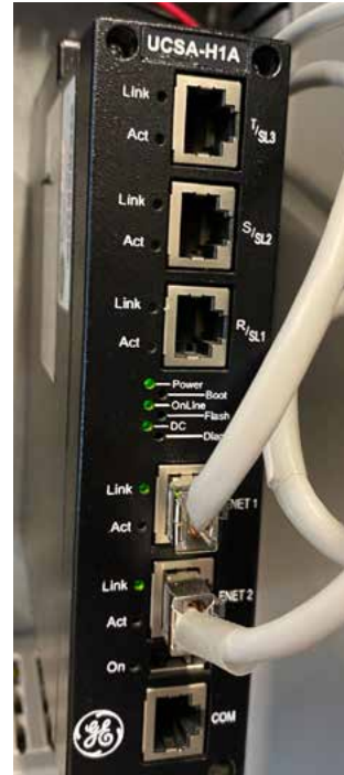
GE Mark VIe Controller (model: IS220UCSAH1A)
